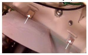
9. Slide the tabs into the slots on the power inlet side of the unit until it locks into place. Replace the 2 ballast mounting screws.
