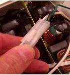
11. Carefully connect the green ground wire to the board. Attach the blue insulated connector to the metal grounding terminal.
