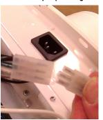
6. Remove the 2 ballast mounting screws then slide the ballast away from the power inlet.
