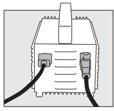
8. Plug ballast into the power supply.
