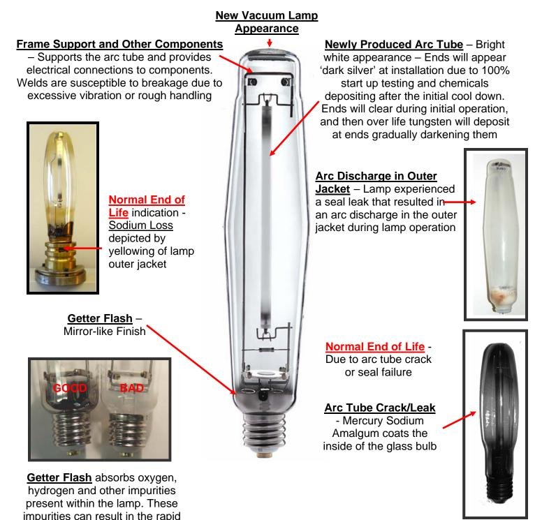
deterioration of the metal parts...resulting in lamp failure
