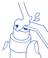
clean the conductivity probe
