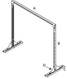
**Step 1.** Place foot over top of outer leg and slide towards bottom.
