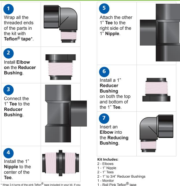
\* Wrap 3-4 turns of the pink Teflon<sup>®</sup> tape included in your kit. If you are using white Teflon<sup>®</sup> tape, wrap 6-8 turns. To wrap, hold the part in your left hand and wrap the Teflon<sup>®</sup> tape clockwise.
