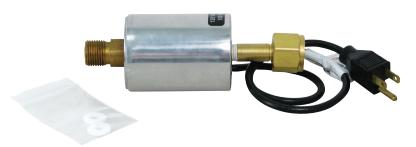
The most economical thermostatically controlled  $CO_2$  heater in the industry, that is designed to prevent  $CO_2$  Regulator freeze-ups. Extends life of  $CO_2$  Regulator and stops  $CO_2$  Regulator diaphragm from freezing. Easily installed between your  $CO_2$  tank and  $CO_2$  Regulator.
