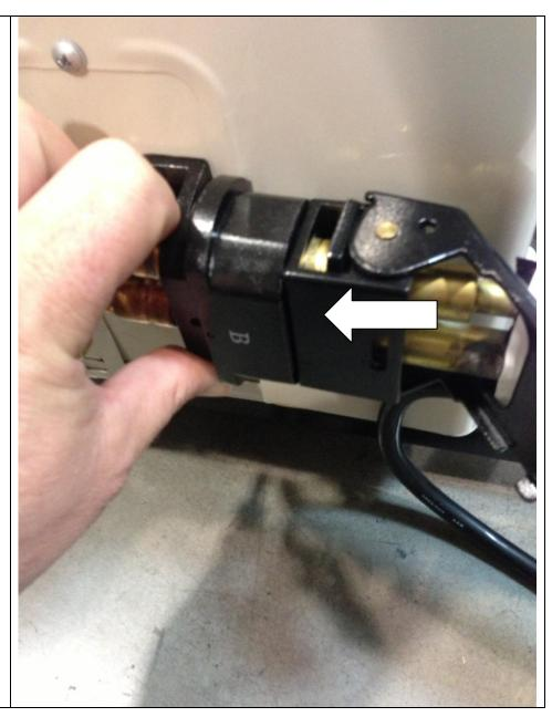
Once connector is in place you must close safety latch completely.
