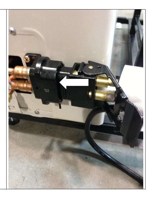
You must insert connector completely into section "B" until it locks into place. A distinct clicking sound will be heard when this is accomplished.
